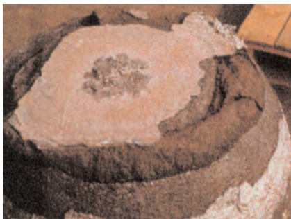
Damage of the crucible chine followed by oxidation in use.
