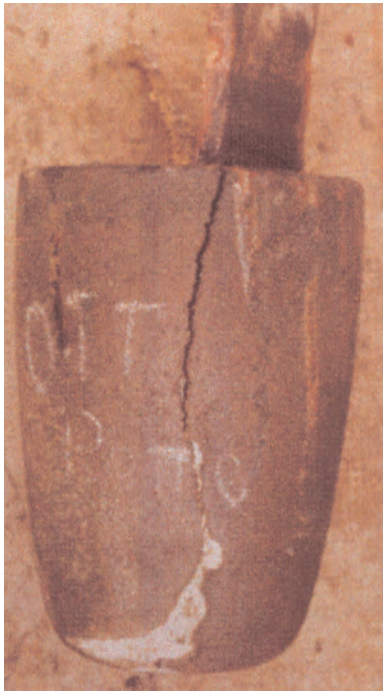
Cracking after subsequent expansion of frozen charge.
