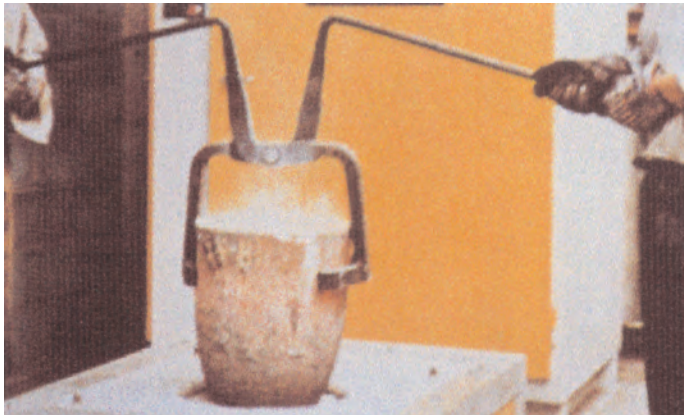
Incorrect use of tongs to lift crucible. The tongs are too high up the body and this causes crushing of the crucible wall.
