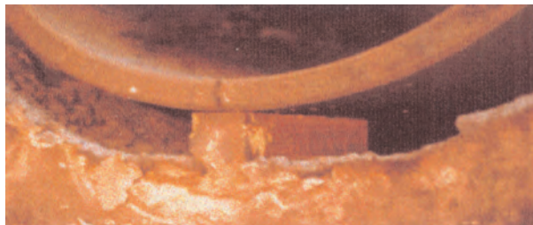
Crucible with cracking showing grip-brick too tight.
