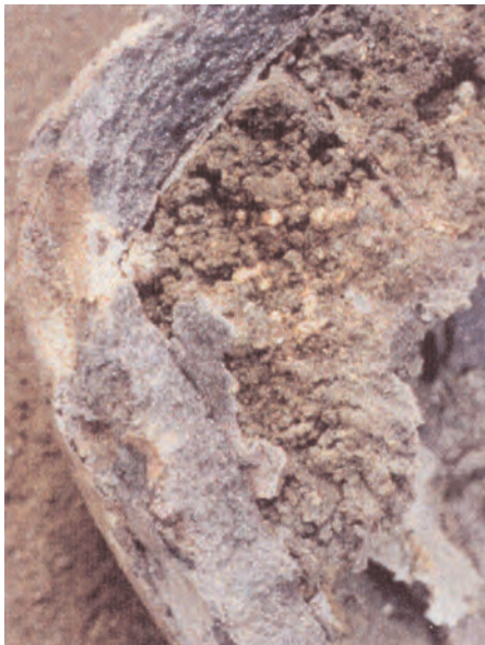
Dross accumulation in the base of the crucible.
