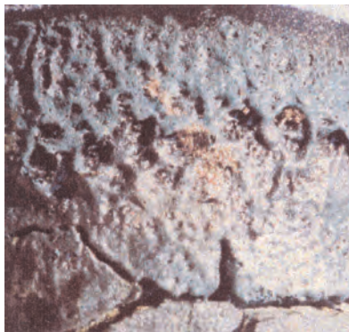
Green, glassy type surface is a clear indication of flux attack.
